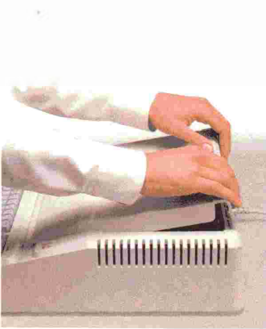
Figure 1-4 Removing the Apple IIe top
