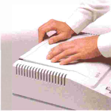
Figure 1-12 Replacing the Apple IIe top
