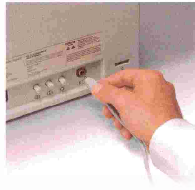
Figure 1-14 Plugging the monitor cable into the monitor
