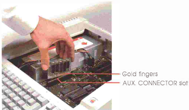
Figure 1-6 Removing the Extended 80-Column Text Card
